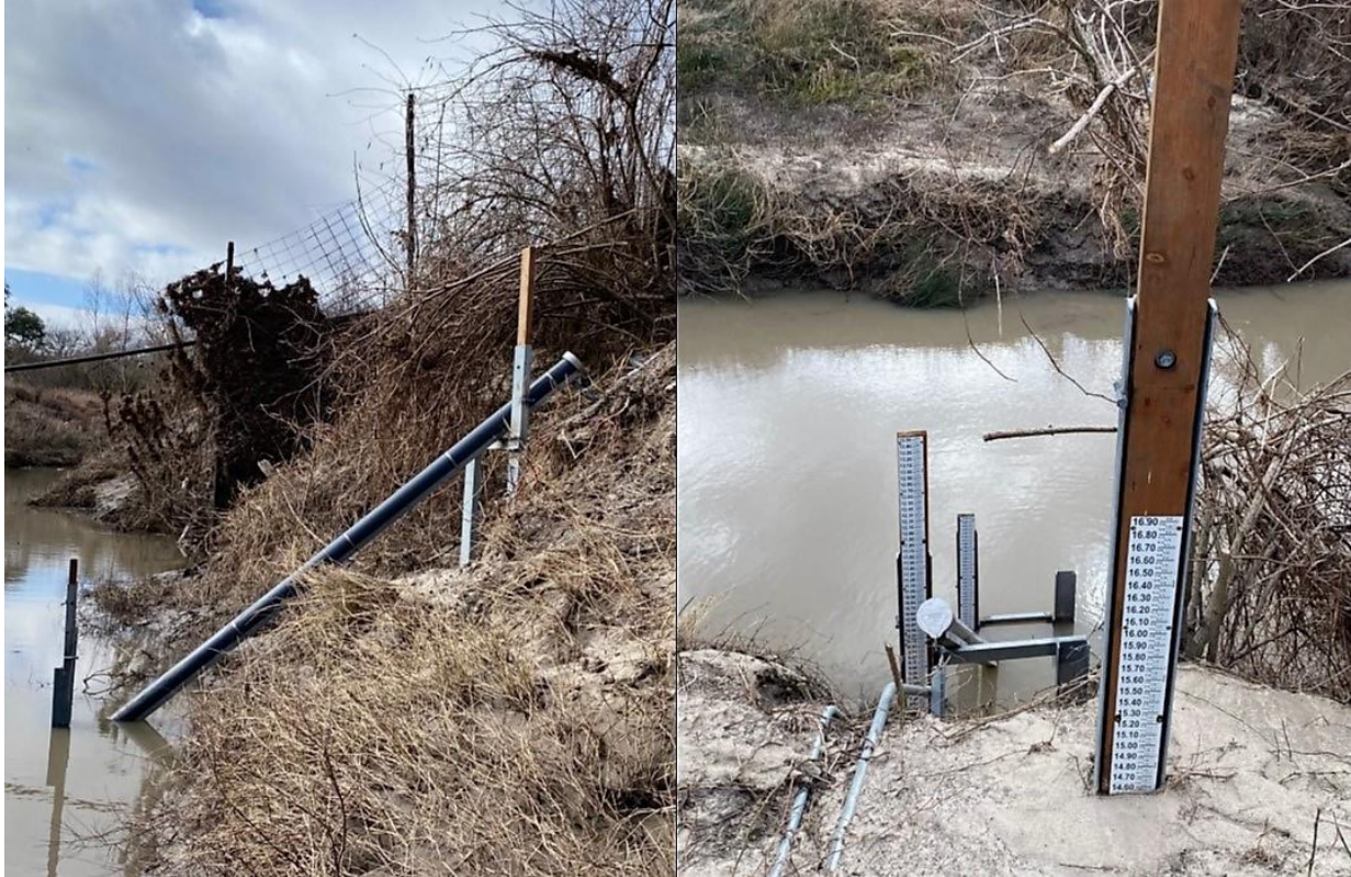
Figure 33: Side View (left) and Top View (right) of the Turbidity Monitor in East Mustang Creek at Station 15382
